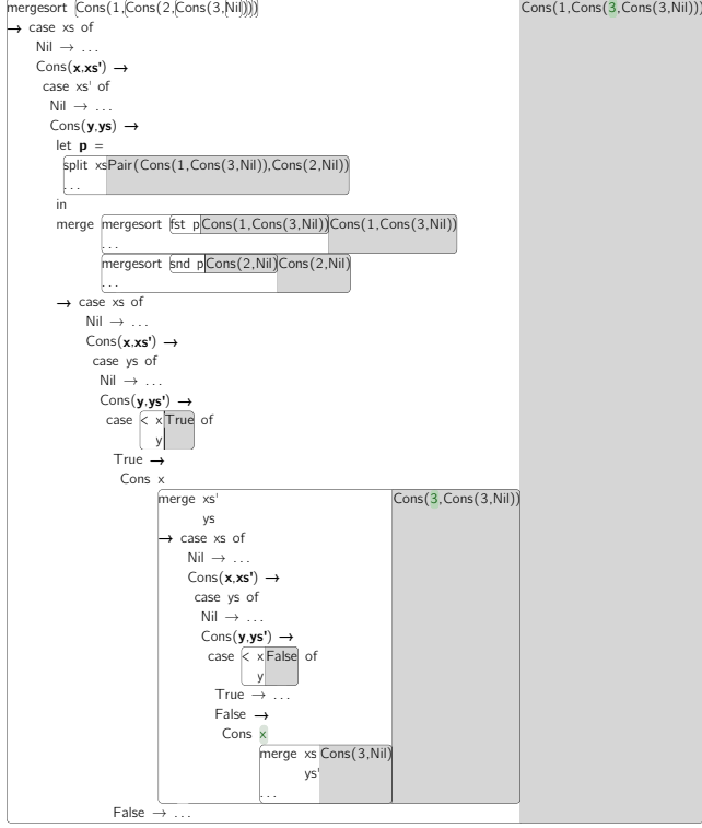
Figure 3. Outermost merge phase of mergesort.
